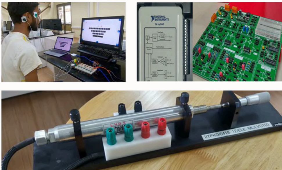
Measurements and Instrumentation Lab, In Clockwise Order from Top: Electro- oculogram EOG Data Acquisition, Analog Signal Conditioning (TI ASLK) and Data Acquisition (NI MyDAQ) and Linear Variable Differential Transformer (LVDT) setup.
