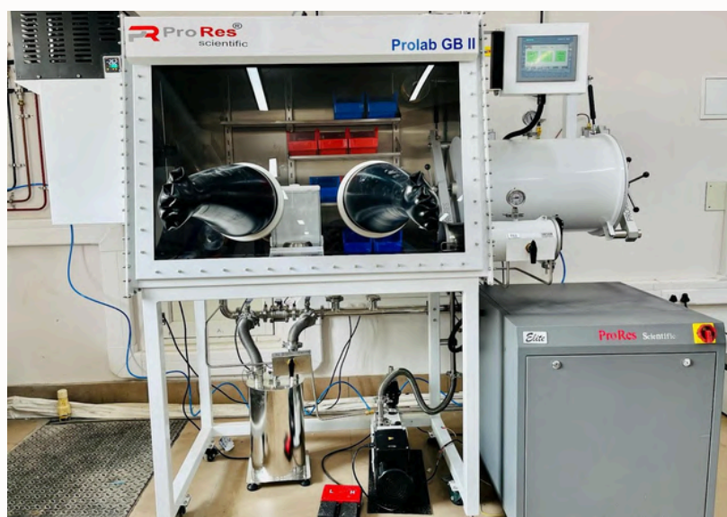
Glove box used for battery applications and to handle highly Air and Moisture sensitive compounds
