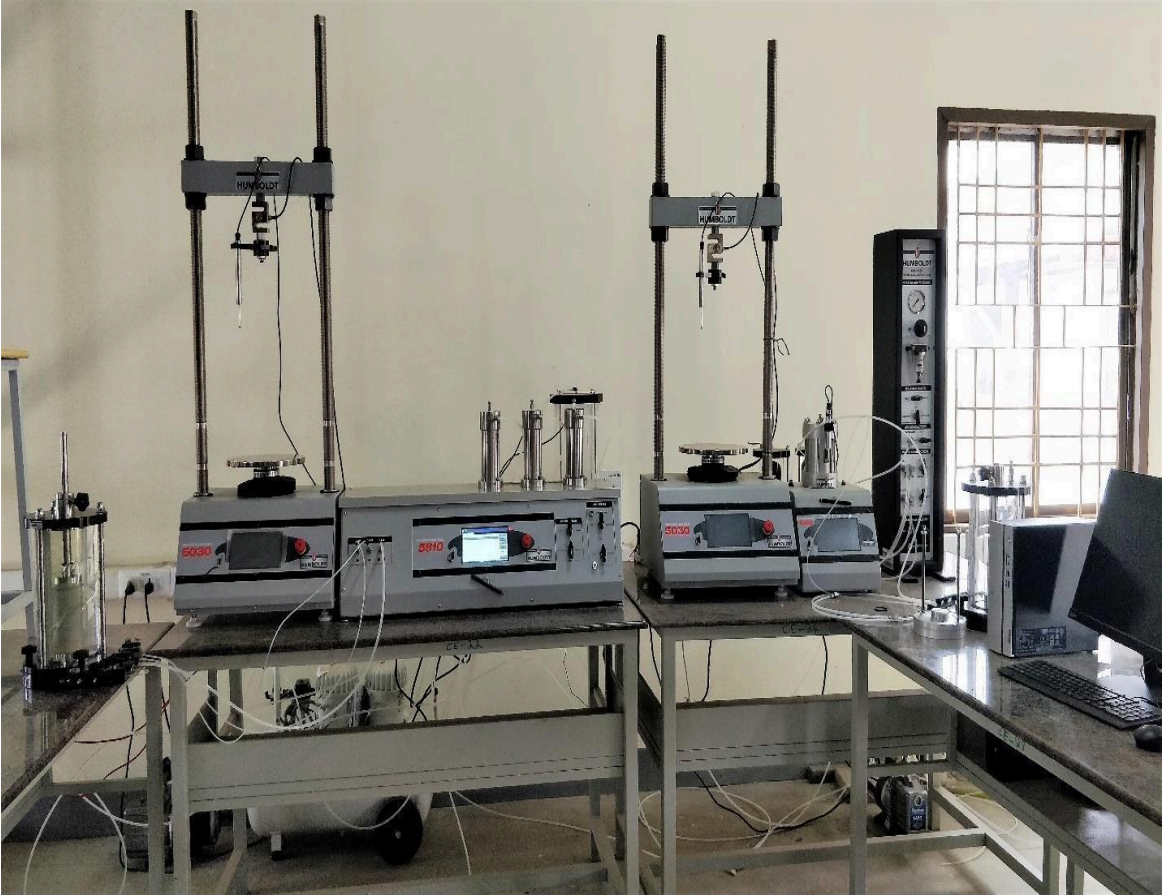
Computerised Static Triaxial System and Flexible Wall Permeameter
