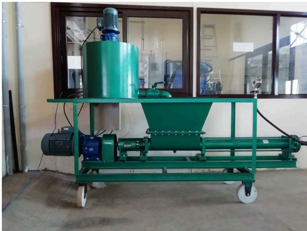
Grout Pump and Sensors for Field Tests
