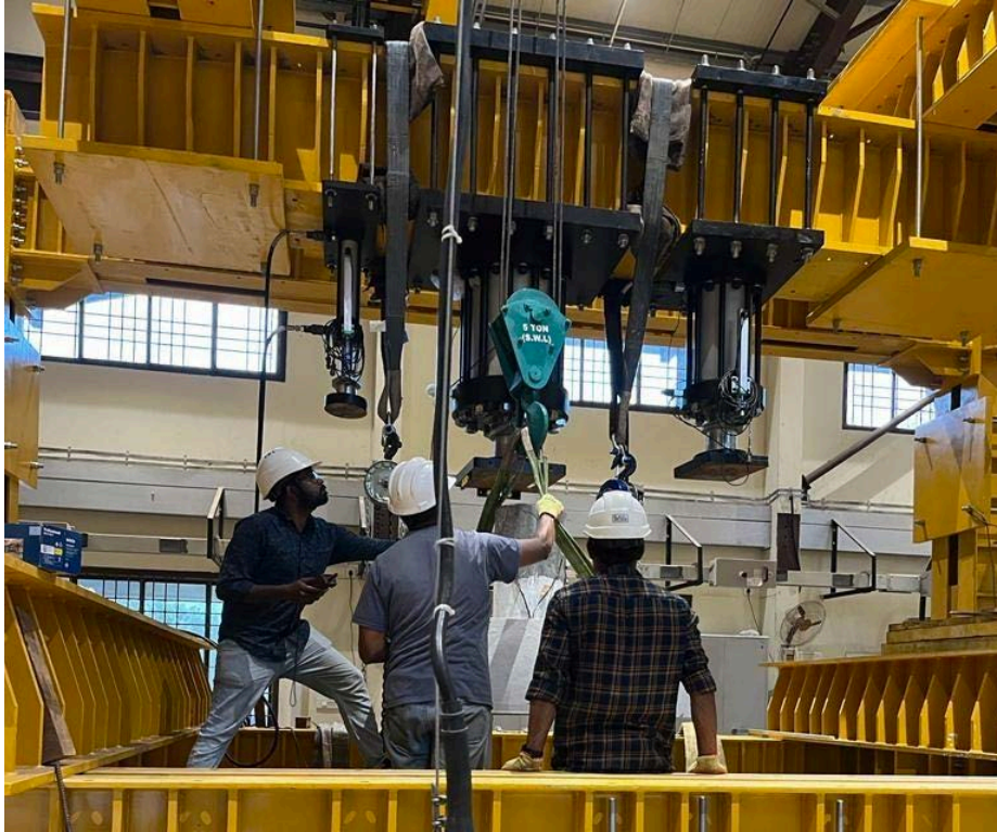
Self-straining test frame having a vertical load capacity of 4000kN and horizontal capacity of 1000kN with Load jacks
