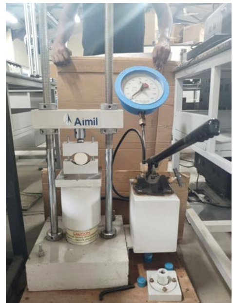
Large Pull Out Test Apparatus for Geosynthetics
