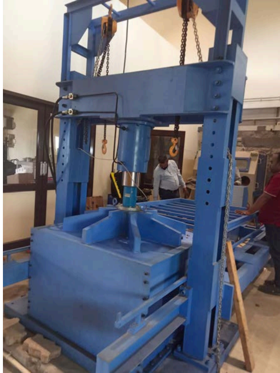
Large Pull Out Test Apparatus for Geosynthetics
