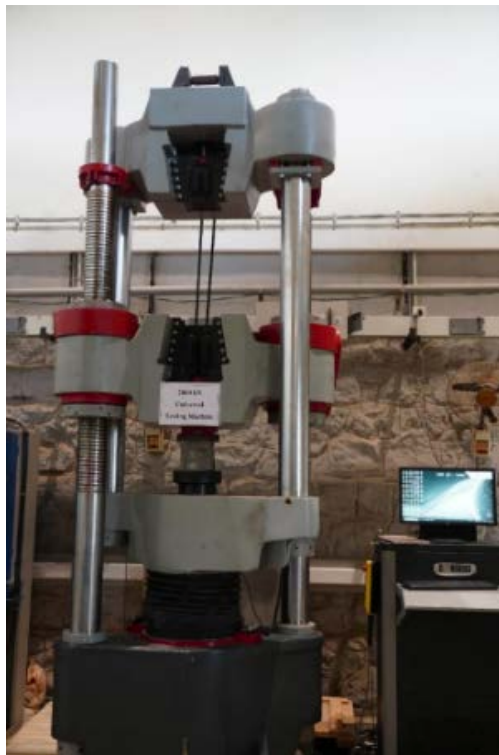
2000kN Capacity Universal Testing Machine
