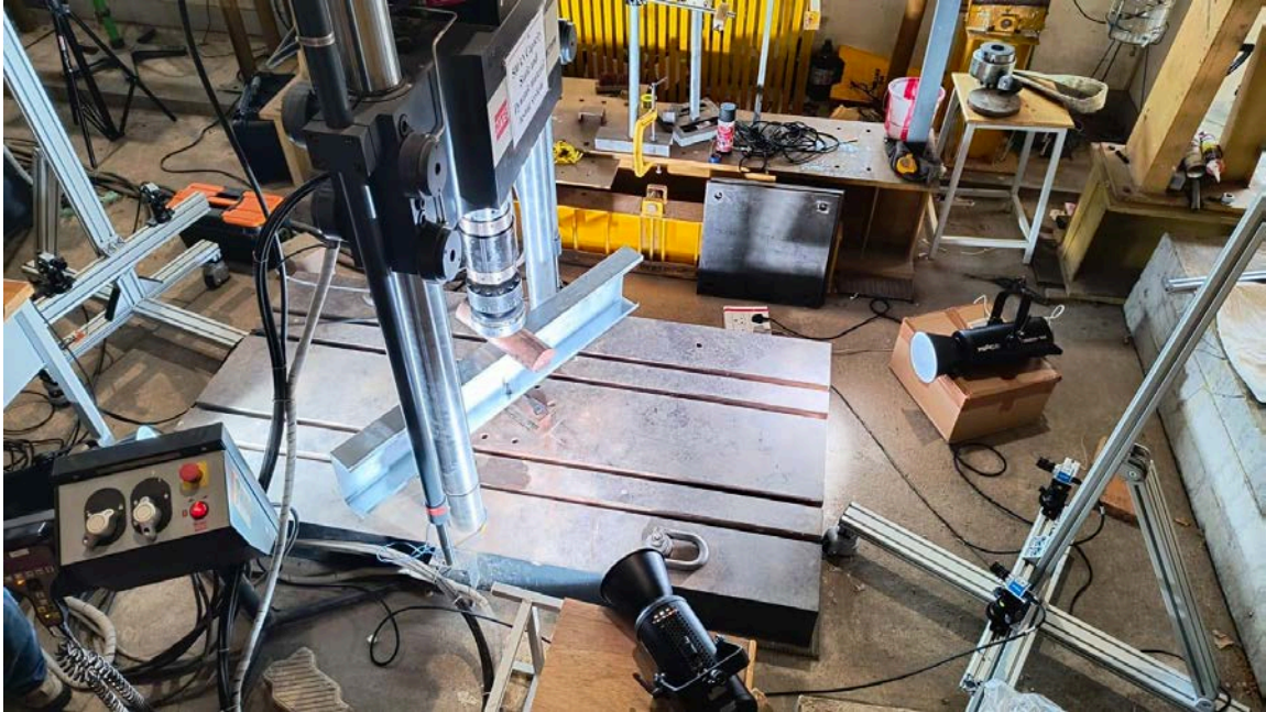
Test Facility Equipped with Digital Image Correlation System
