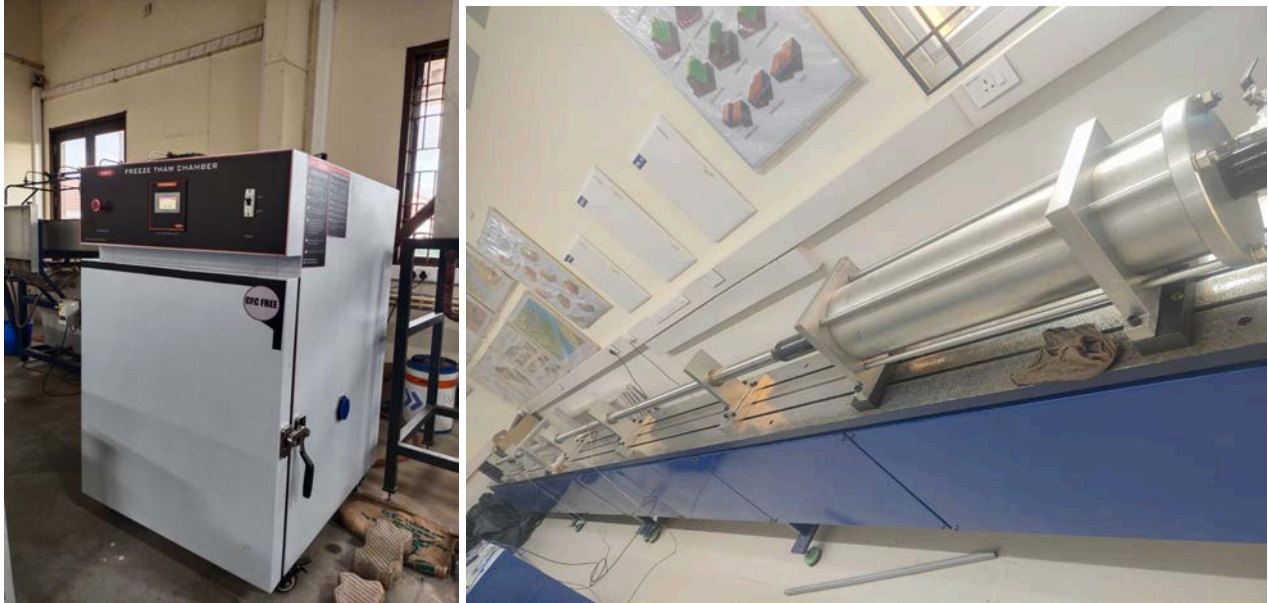
Freezer-Thaw Chamber and Split Hopkinson Pressure Bar (SPHB) Apparatus
