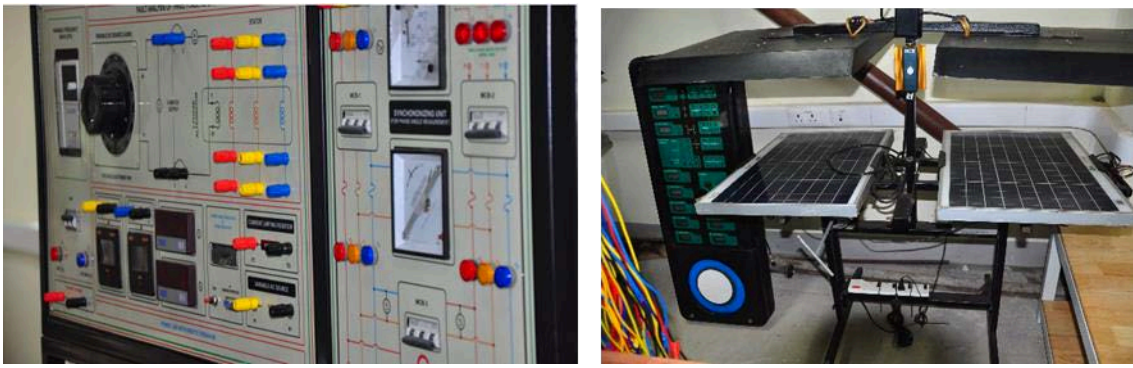
Power Systems Lab, Left: Alternator Fault Simulator With Grid Synchronization Facility, Right: Solar PhotoVoltaic Array Simulator
