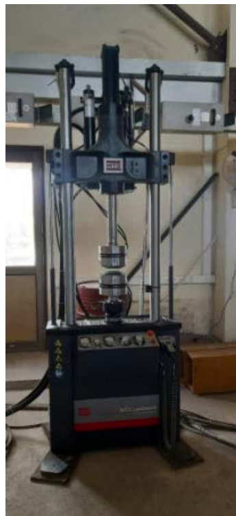
100kN Capacity Servo-hydraulic Static and Dynamic Testing System
