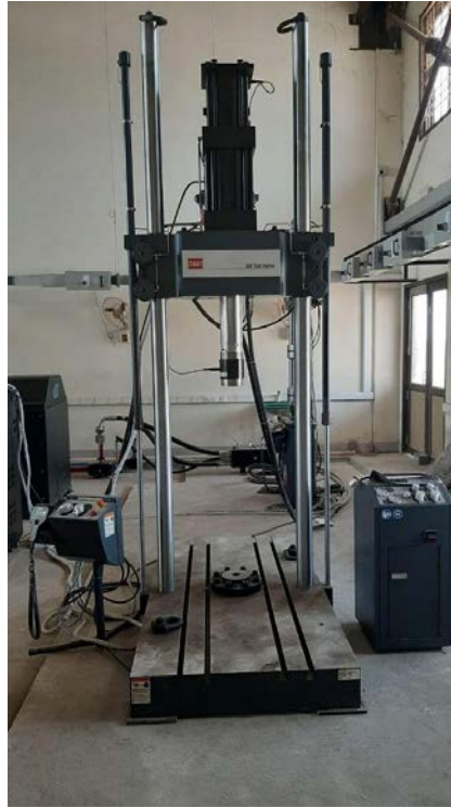
500kN Capacity Servo-hydraulic Static and Dynamic Testing System
