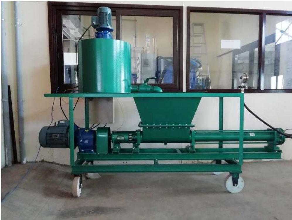
Grout Pump for Field Tests
