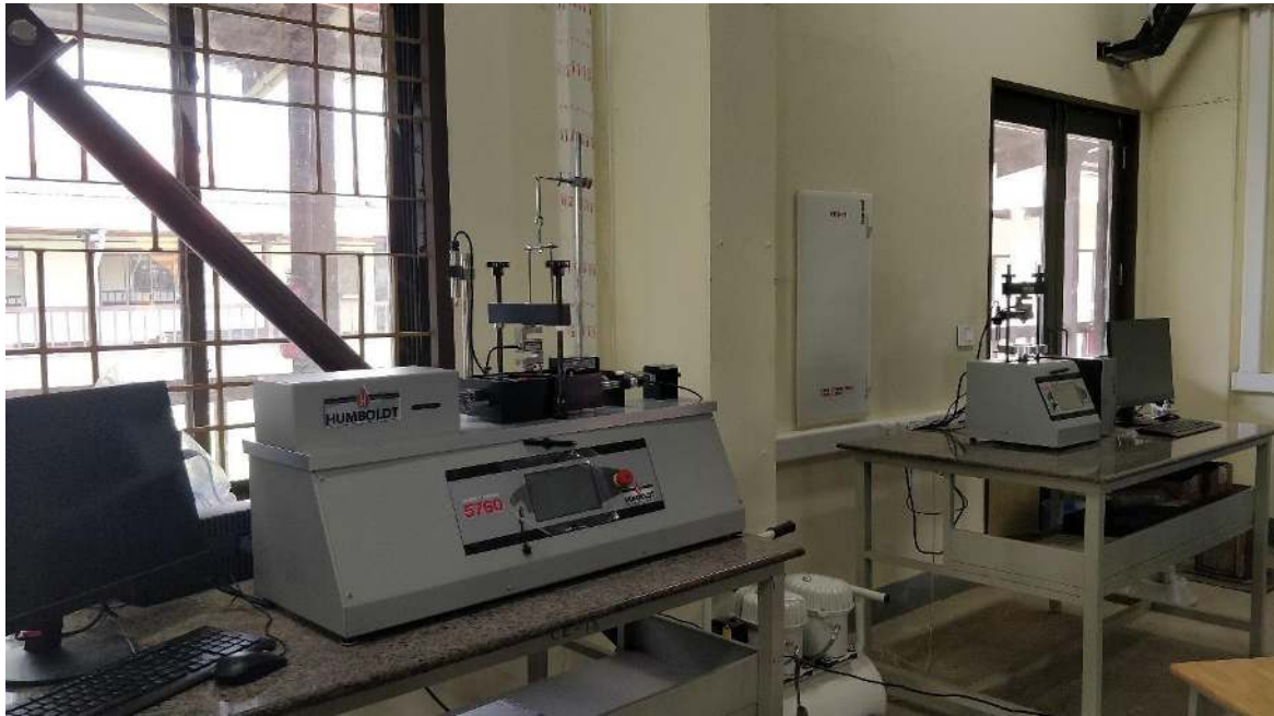
Computerised Static Triaxial System and Flexible Wall Permeameter
