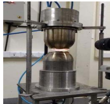
Fig: Opposed jet flame burner
